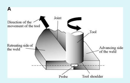
A rotating tool creates heat and plasticizes the metal.
