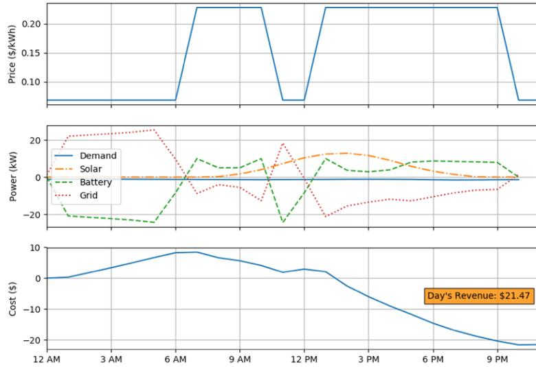
Figure 19: 2 Powerwall Batteries; 70 Solar Modules
