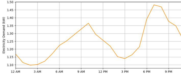
Figure 2: Electricity usage over a 24 hr time period with an average usage of 30kWh
