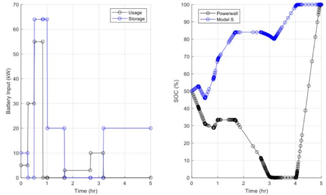
Figure 8: (a) Example of varying the inputs to battery model and (b) transient SOC model output for the Tesla Powerwall and Model S batteries
