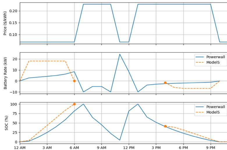
Figure 16: 2 Powerwall Batteries; 70 Solar Modules
