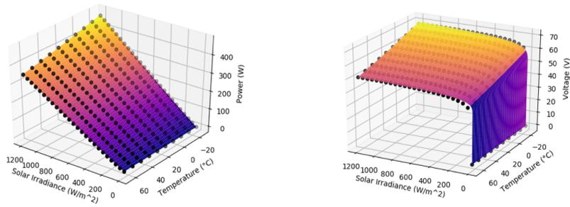
Figure 10: Solar Panel Digital Twin Results
