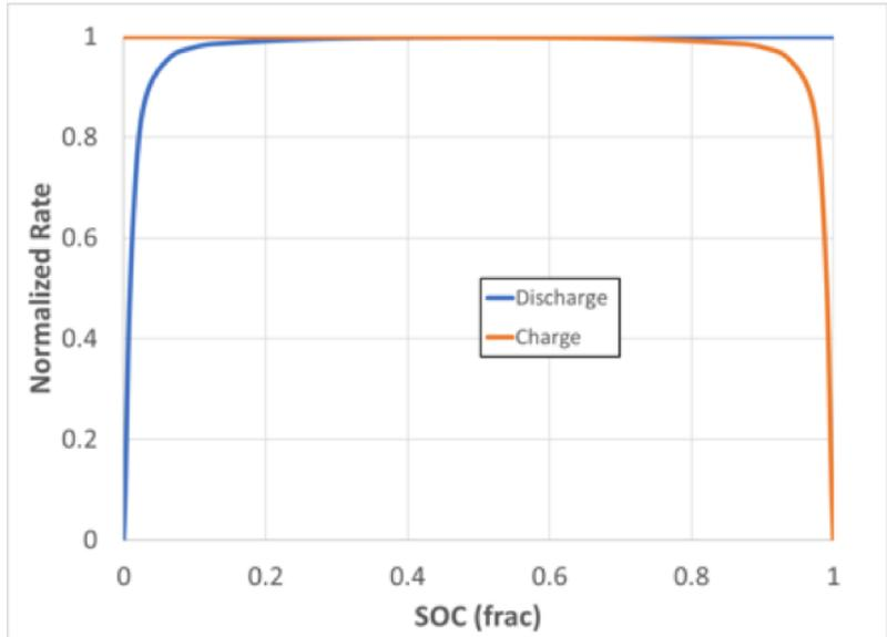
Figure 7: Normalized charge and discharge rates used for simulating the Powerwall and model S batteries
