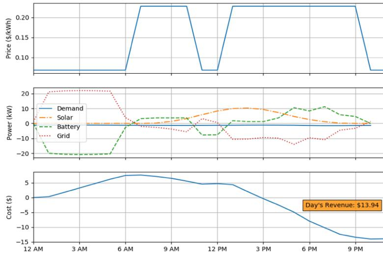
Figure 20: 1 Powerwall Battery; 56 Solar Modules
