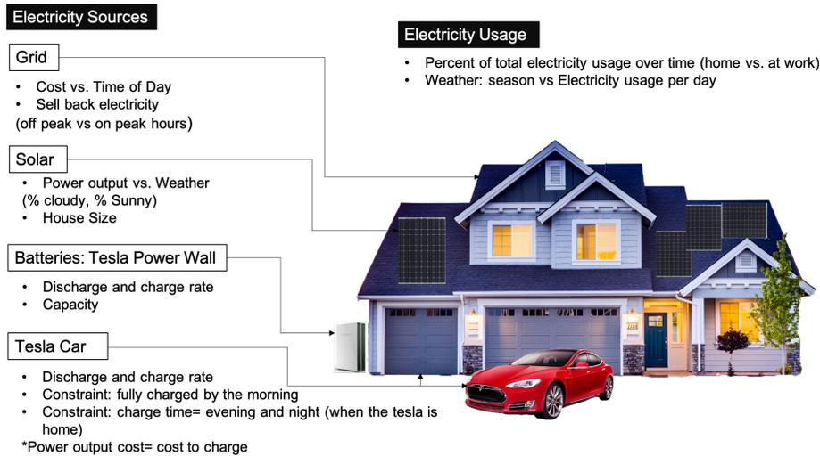
Figure 1: System Diagram
