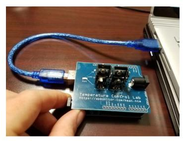
c. Run the following test script to ensure that the device is connected. The LED red light should turn on and then off after 1 second.
