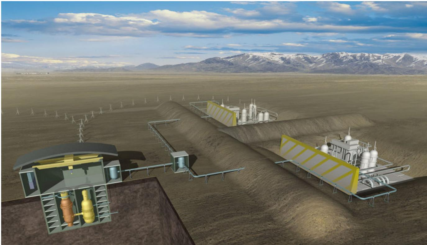
Conceptual nuclear-driven complex for power, hydrogen, and synfuel production
