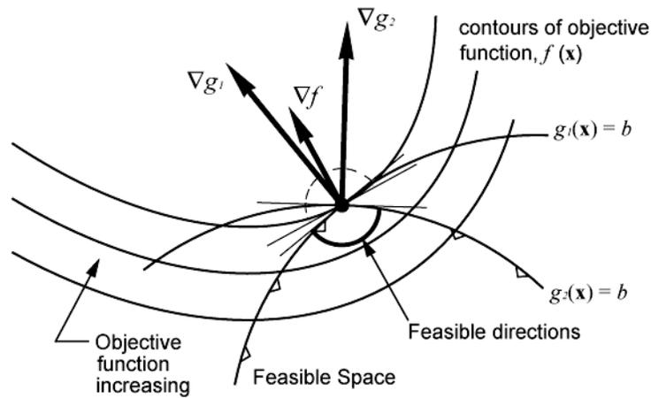
Fig. 7.4 Two binding constraints at an optimum. As long as the objective gradient is within the cone of the constraint gradients, no feasible point exists which improves the objective.
