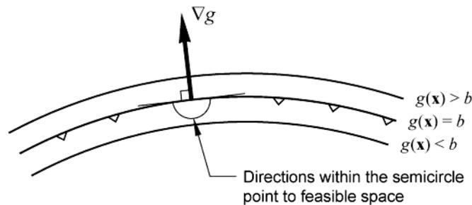
Fig. 7.2 Gradient and set of feasible directions for a constraint.
