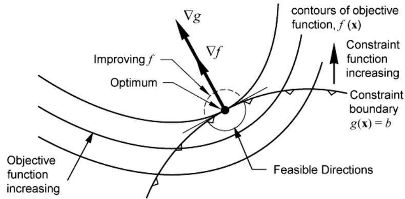
Fig. 7.3 An optimum for one binding constraint occurs when the gradient vectors overlap. When this condition occurs, no feasible point exists which improves the objective.
