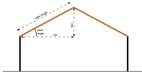
Figure 11: Simple Roof Diagram
