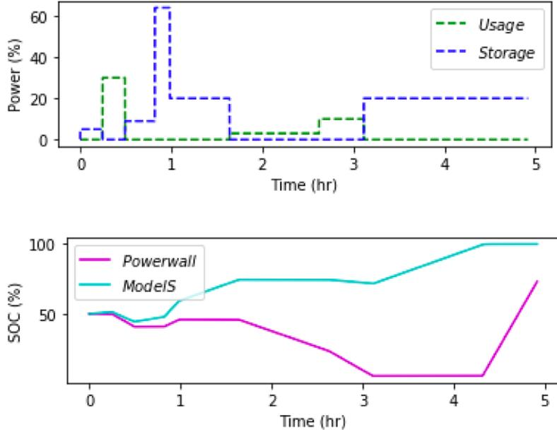
Figure 13: Tesla Car and Wall Batteries with priority on charging the car battery
