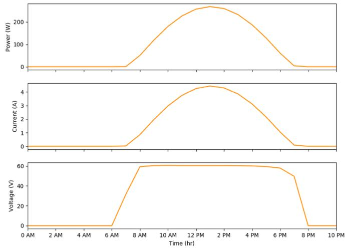
Figure 6: Solar Cell Simulation Output Data
