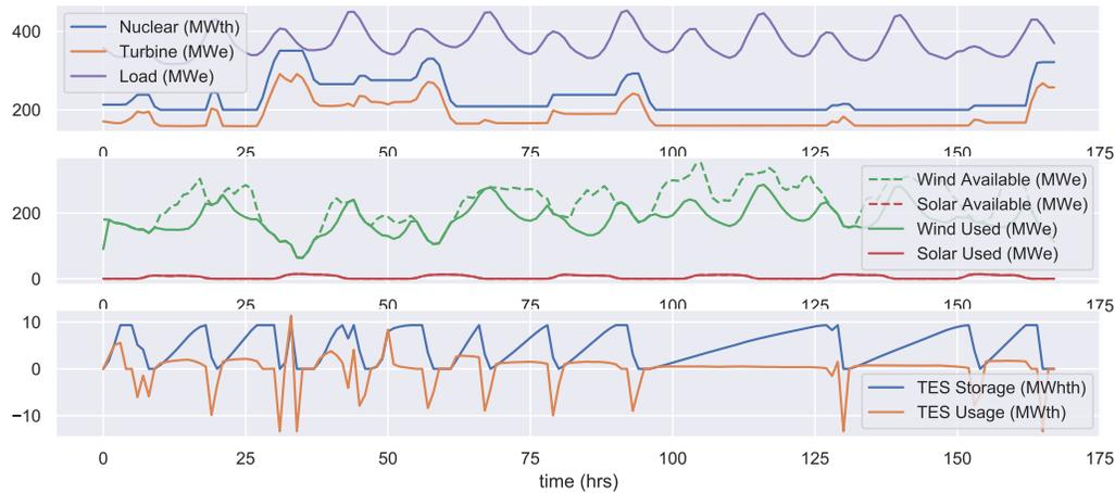
Figure 15: SMR scaling with renewable scaling and curtailment.
