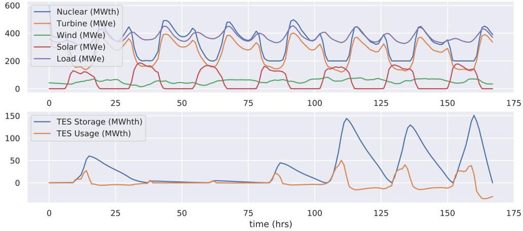
Figure 10: Optimal System Dispatch with DCOST = 0.0
