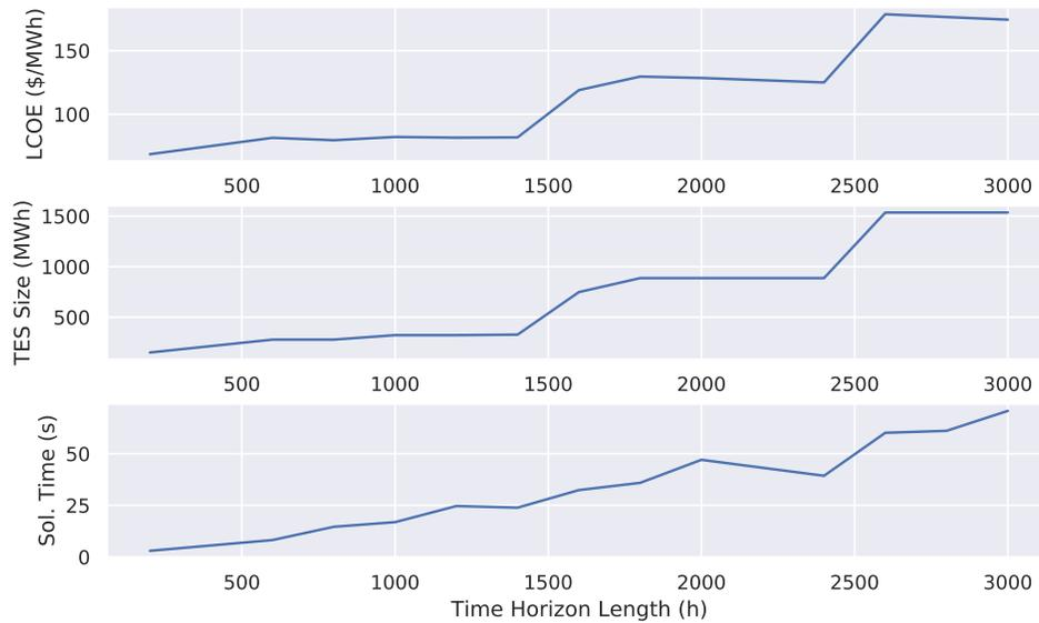
Figure 5: LCOE, TES capacity and solution time variation with increasing time horizon length
