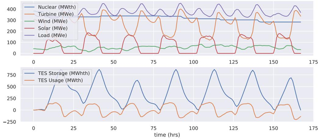
Figure 11: Optimal System Dispatch with DCOST = 0.1
