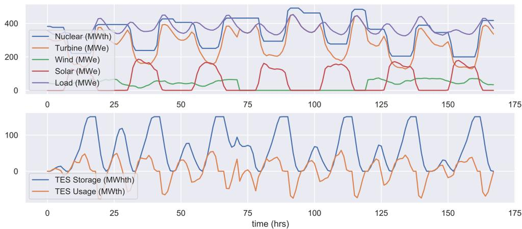
Figure 8: Power Generation Profile with 48 Hours of No Wind Generation
