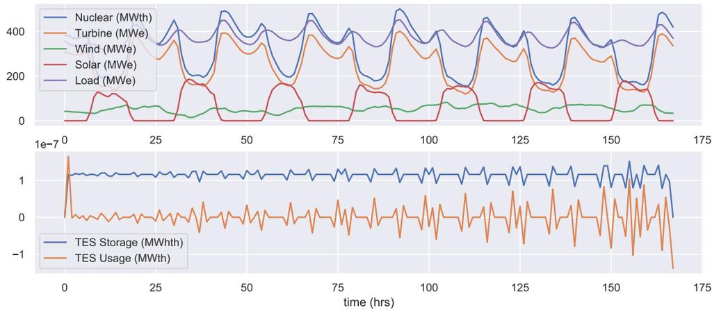
Figure 12: Optimal System Dispatch with No Lower Bound
