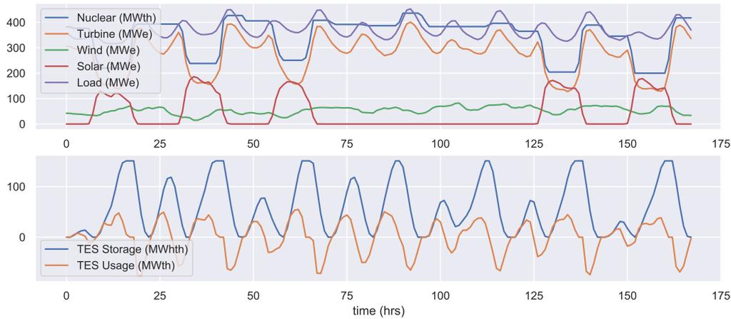
Figure 7: Power Generation Profile with 48 Hours of No Solar Generation
