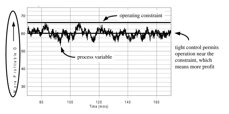
A well controlled process has less variability in the measured process variable, so the process can be operated close to the profitable constraint Profitability of the Process Can Be Improved by Reducing Variability in the Control Loop
